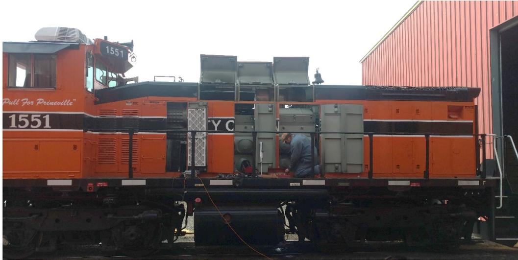
*Injector undergoing replacement in the locomotive at the Prineville Freight Depot*
