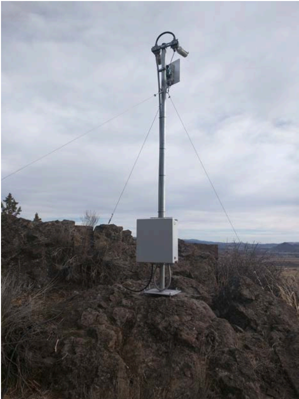
Time lapse camera installed for Wetlands Project
