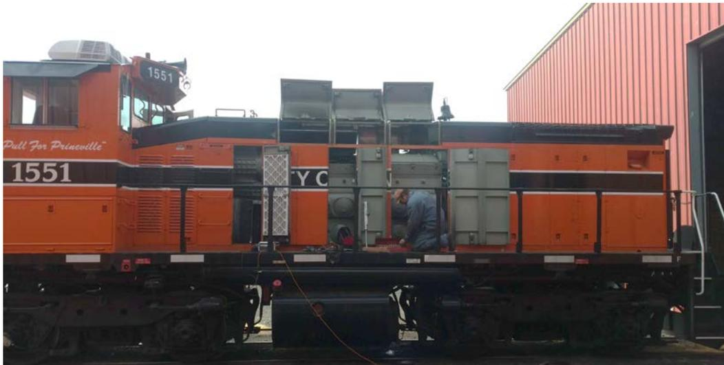
*Injector getting replaced in the locomotive at the freight depot.*
