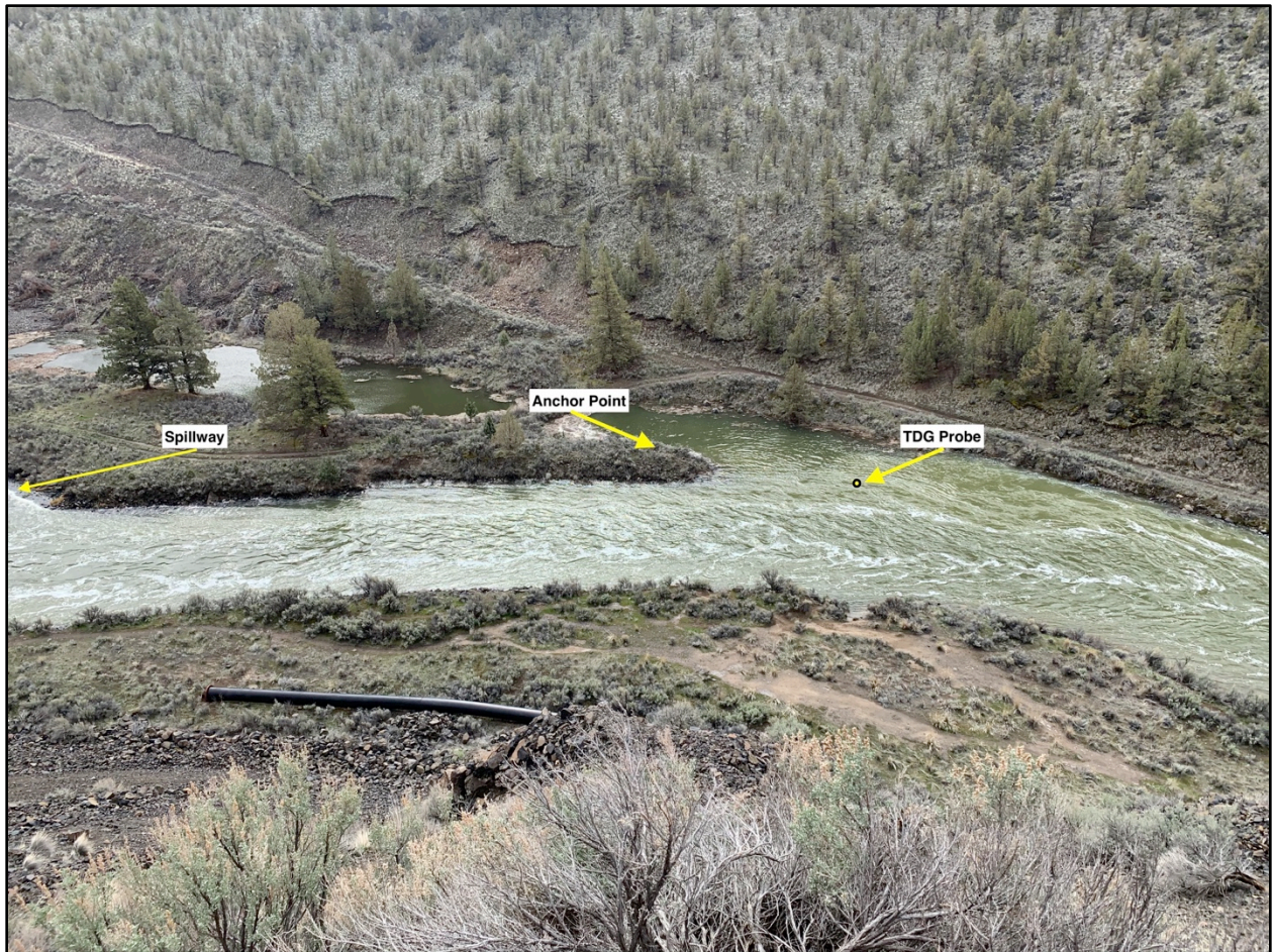
Figure 1. TDG sampling location near Bowman Dam on April 9, 2019 when the flow was 2,900 cfs.
